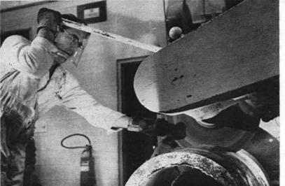
CUT-OFF WHEEL is used by Wilfred Sanchez to cut away the "riser" from the casting. Riser area is always at top of the casting during the pour. Its weight and shape prevent shrinkage.
